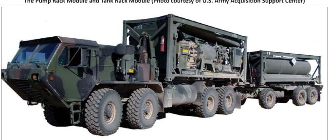
The Pump Rack Module and Tank Rack Module (Photo courtesy of U.S. Army Acquisition Support Center)
