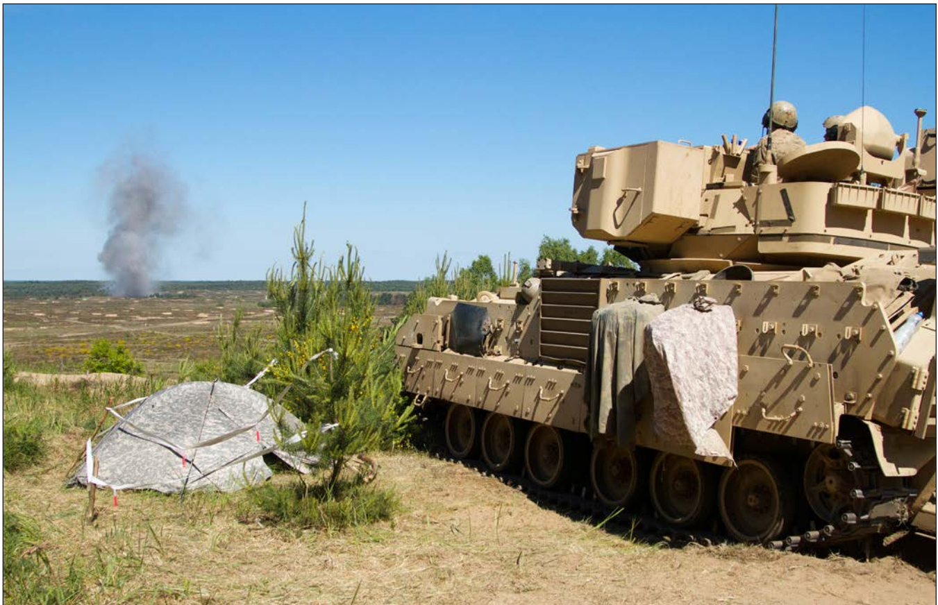
Fire support specialists utilize the M7 Bradley Fire Support Team (BFIST) vehicle and the Fire Support Sensor System (FS3) to identify targets and call for fire (CFF). (Photo by SPC Marcus Floyd)
