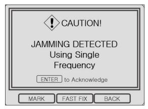
Figure 2 — Example Defense Advanced GPS Receiver (DAGR) Screen
