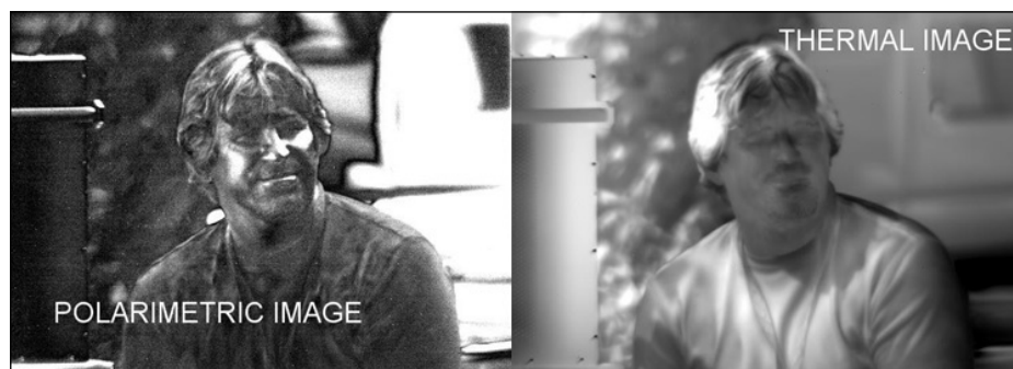
The images above are examples of human identification using conventional and polarimetric thermal cameras. The thermal polarimetric image allows for finer facial details to emerge. (U.S. Army images)
