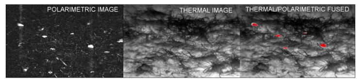
The images above are examples of identification of hidden booby traps and tripwires using conventional and polarimetric thermal cameras.
