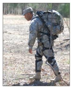
During an energy-harvesting technology demonstration at Fort Devens, MA, Soldiers test a photovoltaic Solar Panel Harvester (left), a kinetic knee harvester (middle), and a backpack frame kinetic harvester (right). (Photos by David Kamm)
