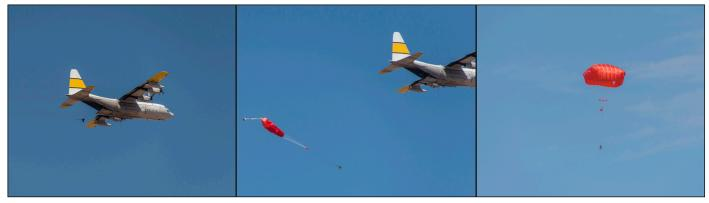
This series of photos shows a simulated towed jumper scenario with a mannequin that is towed behind an aircraft. The Towed Jumper Recovery System includes an emergency parachute that is released once the jumpmaster cuts the aircraft anchor line cable. (U.S. Army photos)
