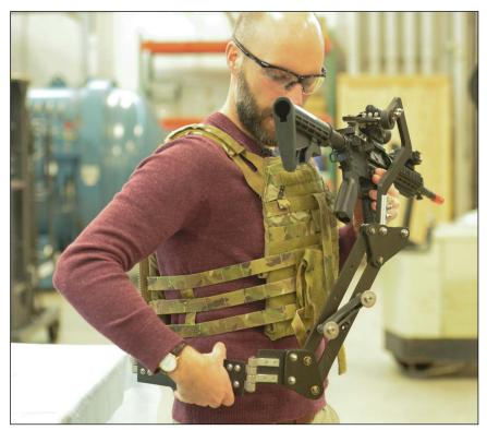
Army Research Lab engineer Dan Baechle demonstrates how to strap on a mechanical device designed to improve Soldiers' accuracy and reduce fatigue.
