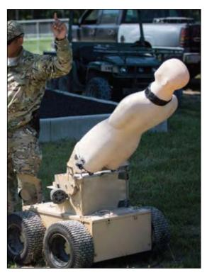
The robotic moving targets used during testing were humanlike, mobile mannequins embedded with pressure sensors to register lethal and non-lethal hits targets.
