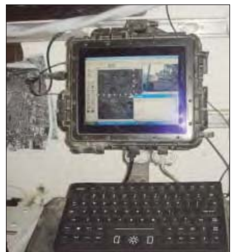
The T-6 ruggedized tablet computer allows the viewing and recording of the UAV video feed.
