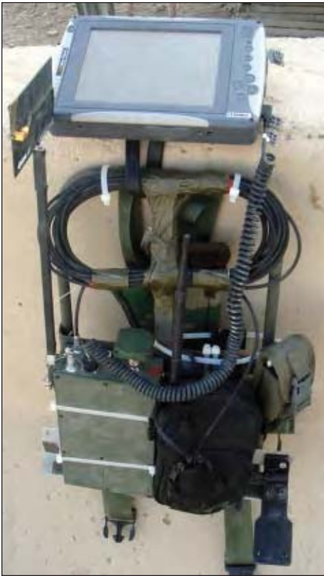
The Ghostbusters pack was developed to make the pilot's combat load more manageable.
