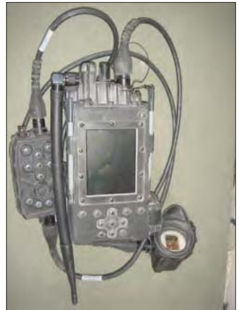
The T-1.5 is a handheld system that can be used to view video and maps, send text messages and conduct voice communications.
