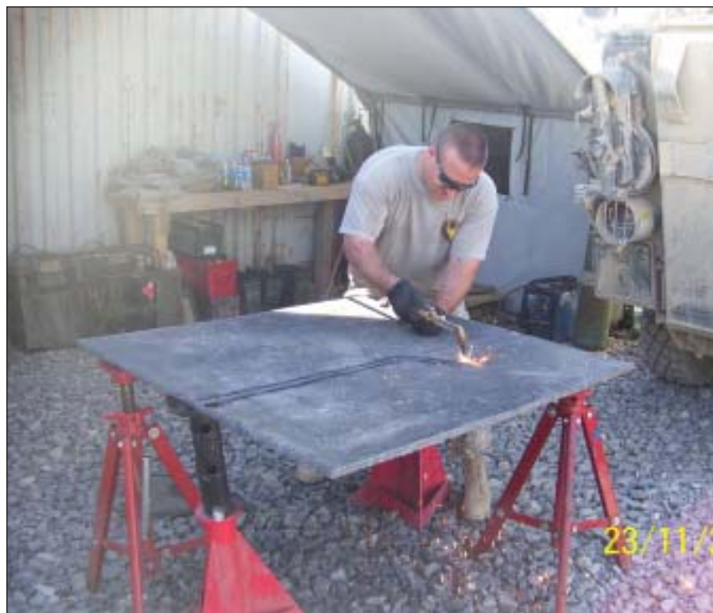
Above, SFC John Giles fills sandbags for firing positions. At right, SFC Steve Steiger cuts steel plate to make F and E-type silhouette targets in preparation for long range carbine marksmanship training.
