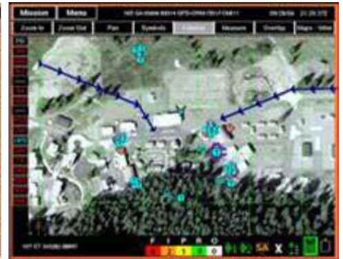
Figure 2 — Views from the Land Warrior common operational picture as seen by the Soldier through the helmet-mounted display. Graphical control measures highlighting a scheme of maneuver (left) and zoom in view of the objective area (right).
