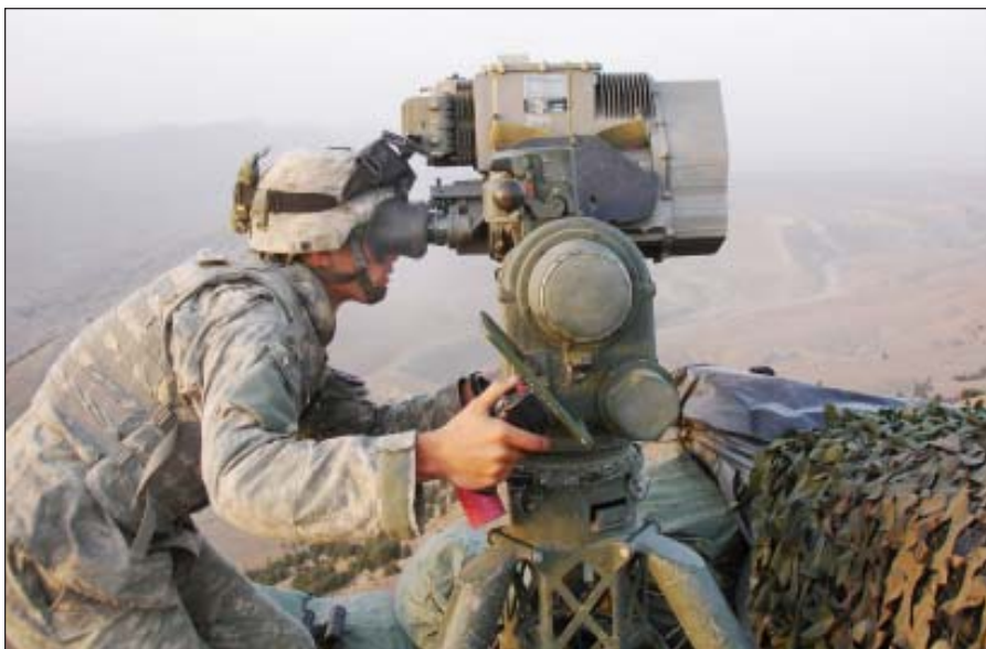
A Soldier with the 2nd Battalion, 87th Infantry Regiment peers across the Pakistani border with the aid of an Improved Targeting Acquisition System from an observation point in Paktika Province, Afghanistan.
