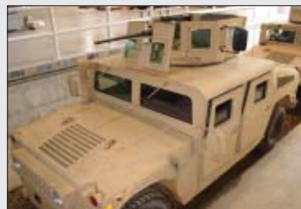
U.S. Army photo A Picatinny Objective Gunner Protection Kit installed on a HMMWV.
