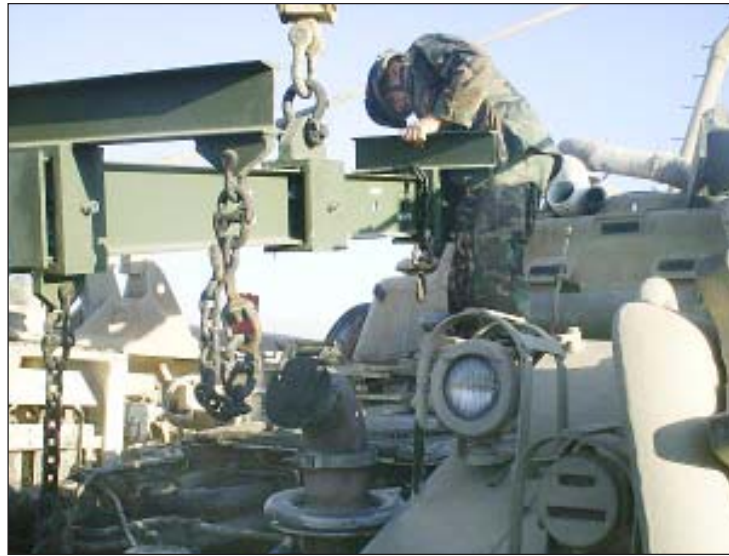
A Soldier with an FSC's Maintenance Platoon replaces an engine on an M88 recovery vehicle.
