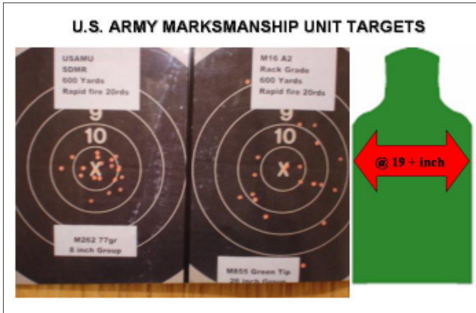
Figure 1 — Technical capabilities: Left target - USAMU-modified M16A4 w/ Mk 262 ammo. Right target - M16A4 w/M855 ammo at 600 yards (9-ring = 20 inches diameter).
