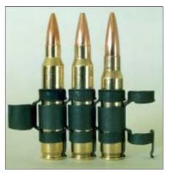
Relatively low cost options for improving performance of 5.56mm weapons are the 5.56x45mm "heavy ball" (left), 6x45mm (center), and 6x41mm (right) cartridges. All three are compatible with 5.56x45mm magazines and bolts as well as the metallic links used to feed the M249, which would greatly simplify the conversion process.
