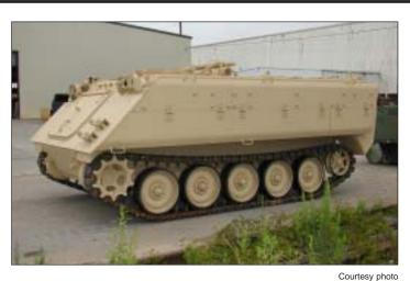
Using the modified Bradley A0 armor would be one way to significantly upgrade the protection level of the M113A3 at a low cost.
