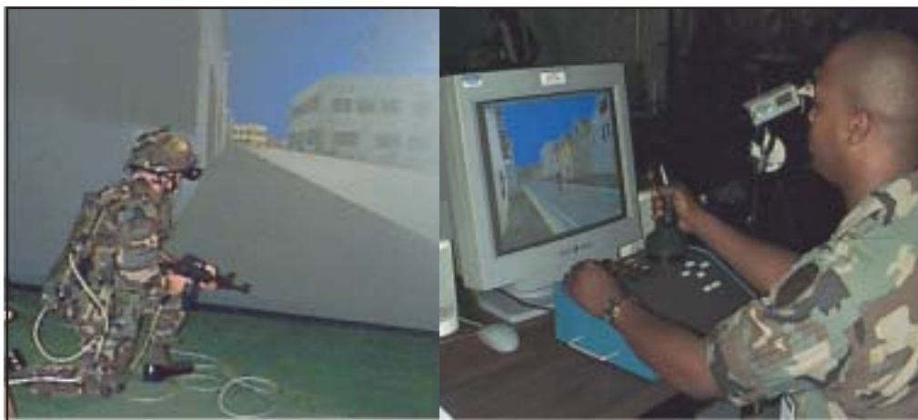
The Squad Synthetic Environment is comprised a fully immersed environment, which is also called stand up (at left) and desktop computer mode (right).
