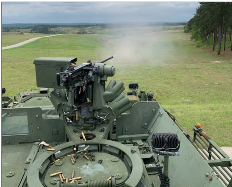
Above, Stryker Leaders Course students engage targets using the Remote Weapon Station-controlled M2 .50 caliber machine gun. (Photo by SSG Tom Emmanuel)
