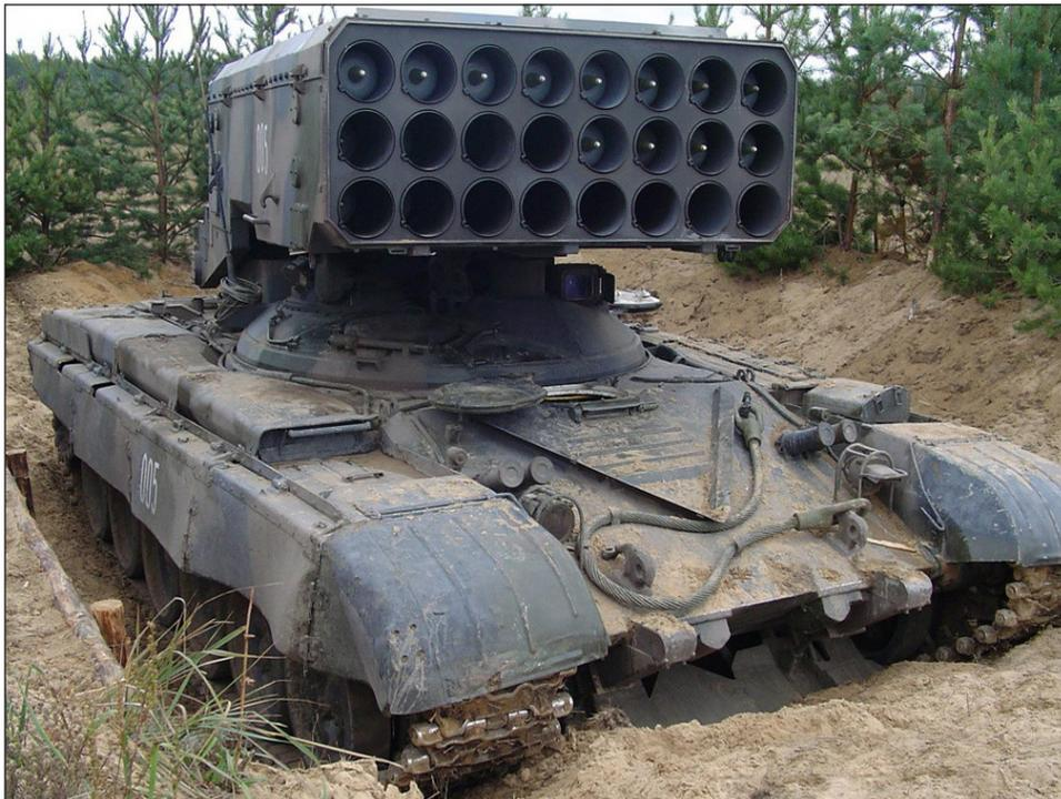
Figure 1 — Russian TOS-1A Solntsepek 220mm Heavy Flamethrower System
