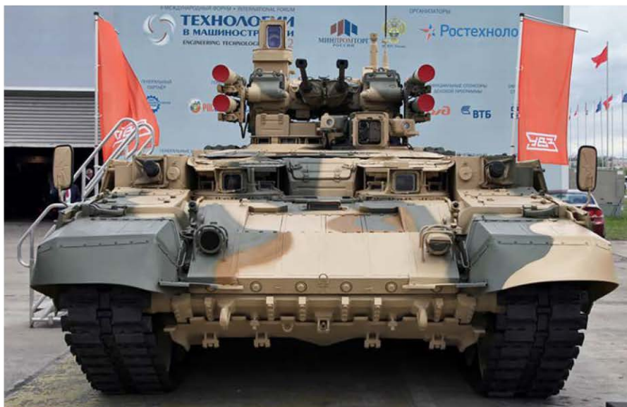
Figure 1. The first model of BMPT-72. Note the unarmored ATGM tubes, hull-mounted grenade launchers above the tracks and Active Protection System tubes barely visible at the base of the turret. (Photo copyright Vitaly Kuzmin. Licensed under a Creative Commons Attribution-NonCommercial-NoDerivatives 4.0 International License.)
