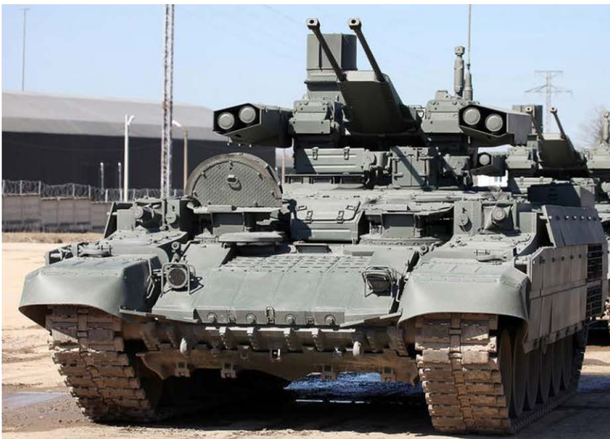
Figure 6. The Russian Army BMPT-72. Note that the turret has been modified with armor surrounding the ATGM tubes and some other changes, but the hull retains the grenade launchers. (Photo copyright Vitaly Kuzmin. Licensed under a Creative Commons Attribution-NonCommercial- International License NoDerivatives 4.0.)
