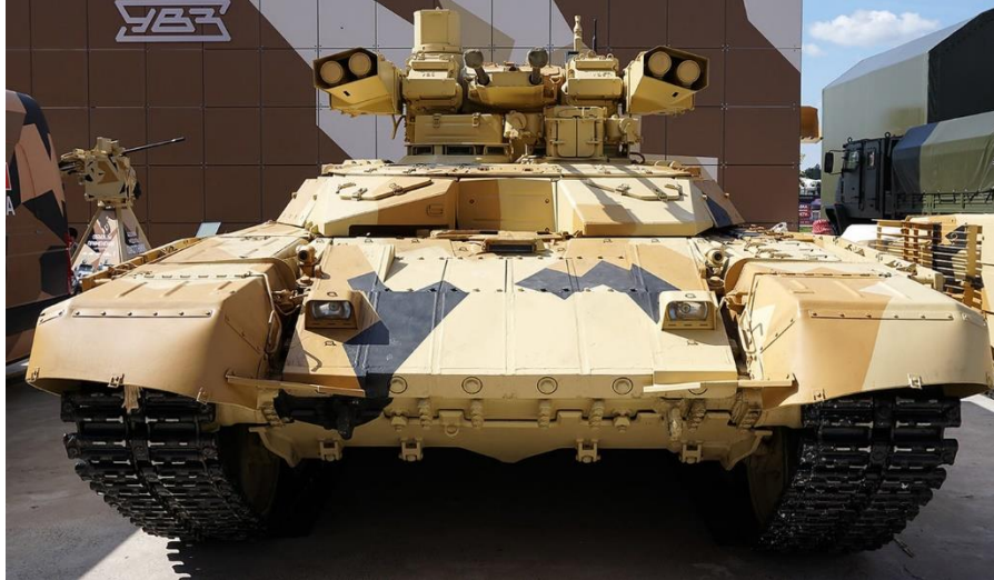
Figure 4. The latest model of BMPT-72 destined for the export market. Note the redesigned turret and lack of forward-facing grenade launchers. (Photo copyright Vitaly Kuzmin. Licensed under a Creative Commons Attribution-NonCommercial-NoDerivatives 4.0 International License.)
