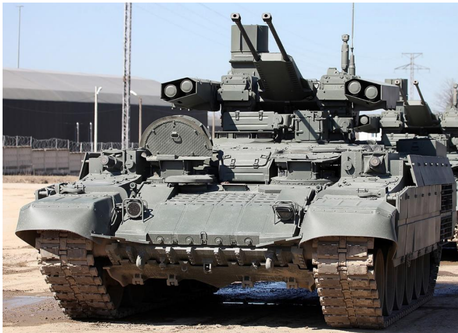
Figure 6. The Russian Army BMPT-72. Note that the turret has been modified with armor surrounding the ATGM tubes and some other changes, but the hull retains the grenade launchers. (Photo copyright Vitaly Kuzmin. Licensed under a Creative Commons Attribution-NonCommercial- International License NoDerivatives 4.0.)
