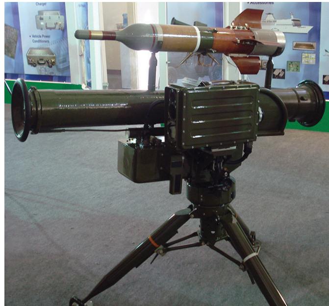
Figure 3. The Baktar-Shikan ATGM, a licensed-manufactured variant of the HJ-8 (or Hongjian-8, translated as Red Arrow-8), is a second-generation TOW anti-tank missile system originally deployed by the Chinese People’s Liberation Army. Pakistan produces this missile system under license as the Baktar-Shikan. (Photo from Wikipedia; used under license)
