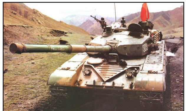
Elevated view of the Type 98 reveals details of the box-like turret roof, new optics for the commander and gunner, and the triangular lifting eyes along the turret upper edge. The Laser Self-Defense Weapon can be seen on the gunner's left.
