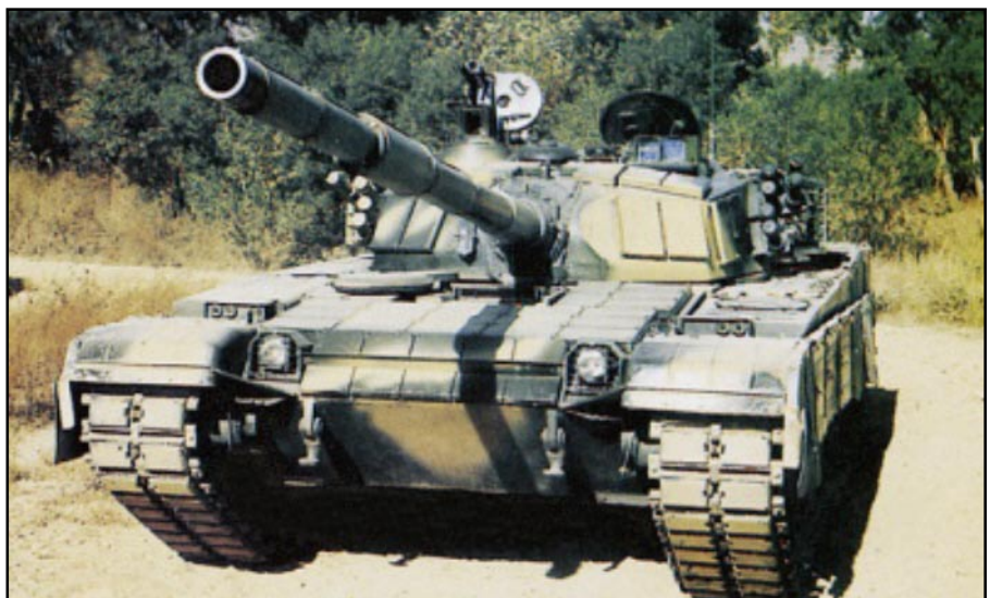
The earlier Type 90II/Type 90 IIM, seen here in a manufacturer's brochure with simulated add-on armor, did not meet China's expectations, but may be built for export.
