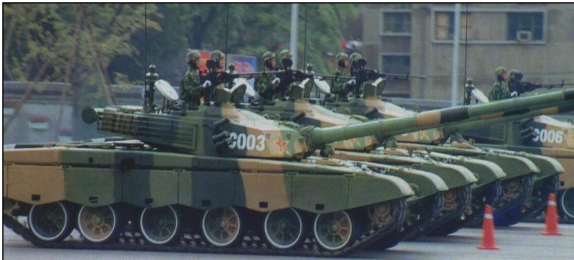
Chinese Type 98 MBTs on parade in Beijing in October. Note new hull skirts, rubber padded tracks, and the raised turret roof.
