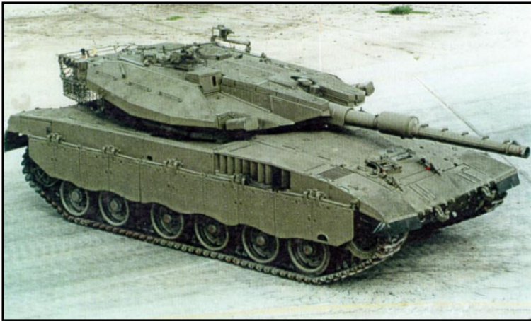
This Merkava Mk.3 has been upgraded with modular armor suite and thermal sleeve integrated into the main gun barrel. At right, a view of the rear hull door, useful for MEDEVACing casualties and as an escape hatch for the crew.
