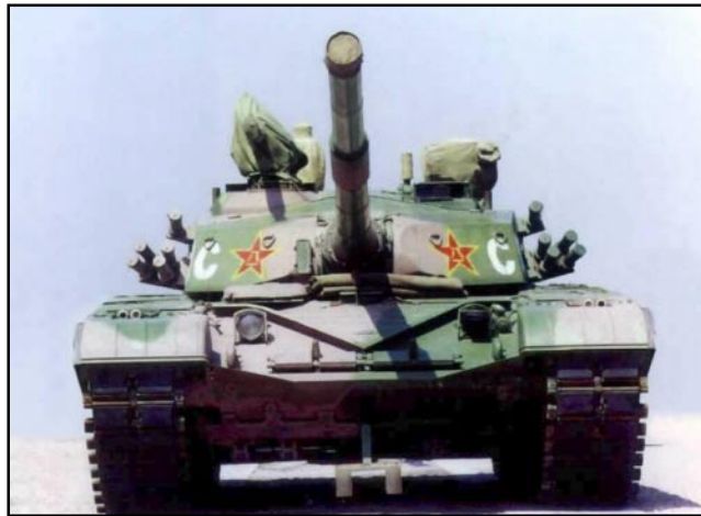
The New Chinese Type 98 – Configuration of the turret roof, from left, includes the covered commander's machine gun, the Laser Warning Receiver, wind sensor, and the Laser Self-Defense weapon.
