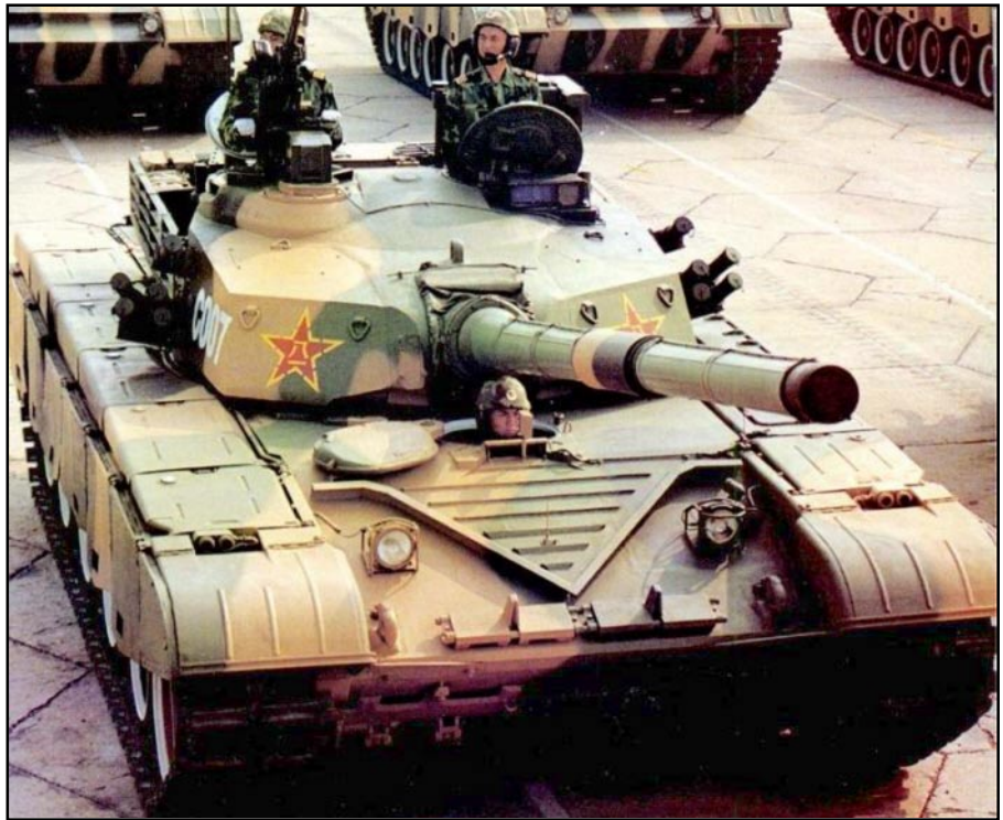
Elevated view of the Type 98 reveals details of the box-like turret roof, new optics for the commander and gunner, and the triangular lifting eyes along the turret upper edge. The Laser Self-Defense Weapon can be seen on the gunner's left.
