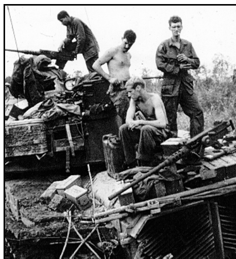
Above, at left, a 7.62mm Minigun salvaged from a helicopter was mounted in front of the loader's hatch... until the crew was ordered to remove it.
