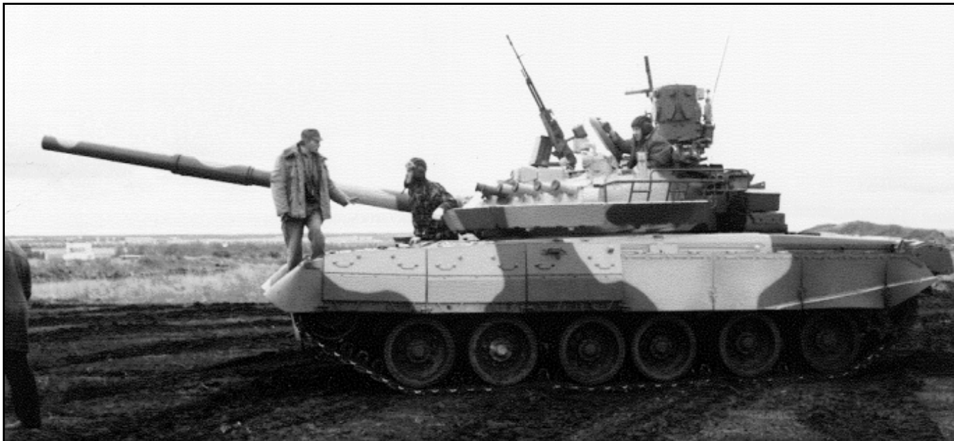
Elements of the Arena Active Protection System include ring of explosive panels at lower margin of turret ring and radar on turret roof.
