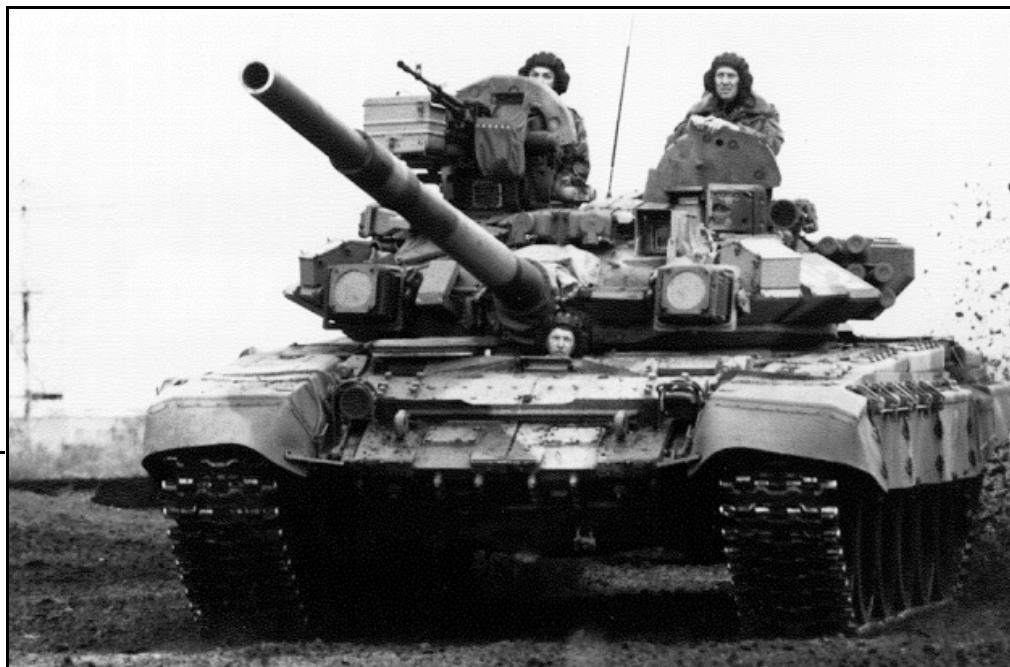
The Shtora system jammers are the two boxes at either side of the gun tube. Grenade dischargers are at the rear of the turret.
