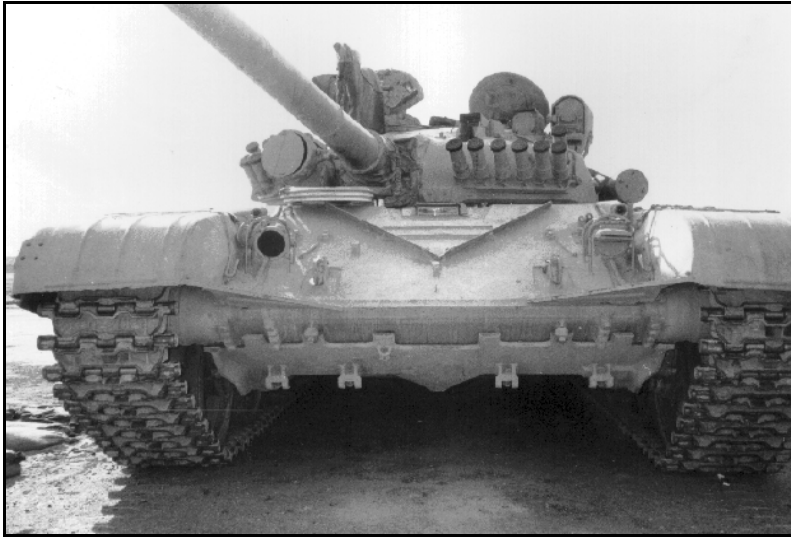
An early — and unsuccessful — attempt at a countermeasure to missiles like the TOW and Dragon, these infrared “dazzlers” (above) were discovered on Iraqi tanks in DESERT STORM.
