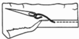
Figure 3. Turn Edge Under and Sew.
