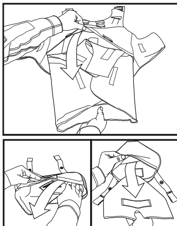
Figure 5. Removing Soft Ballistic Inserts.
