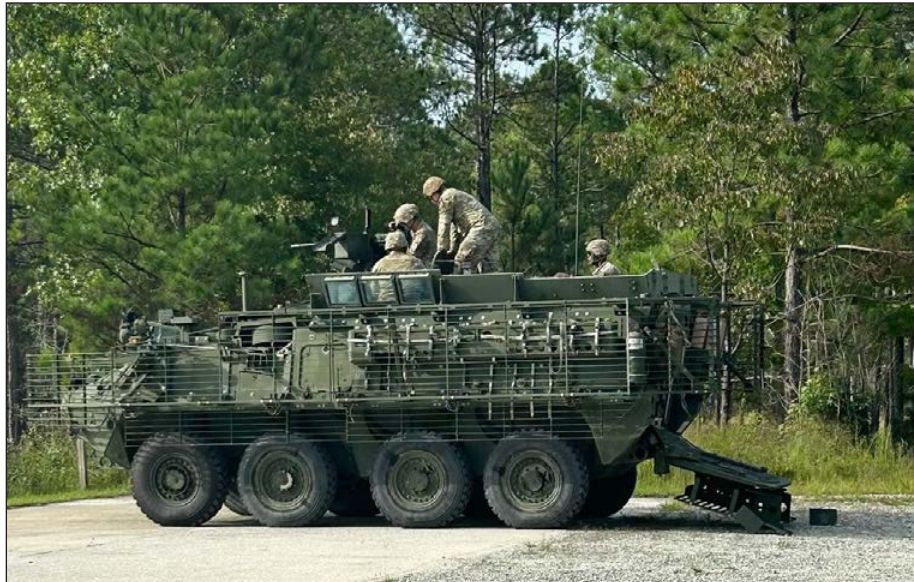
Students in the Stryker Leader Course prepare to conduct a live-fire familiarization of the Stryker Infantry Carrier Vehicle's Remote Weapon Station (RWS) at Ruth Range. During the exercise, students engage a variety of targets with RWS-mounted M2A1 .50 caliber machine guns and MK19 40mm automatic grenade launchers. (Photo courtesy of SLC)
