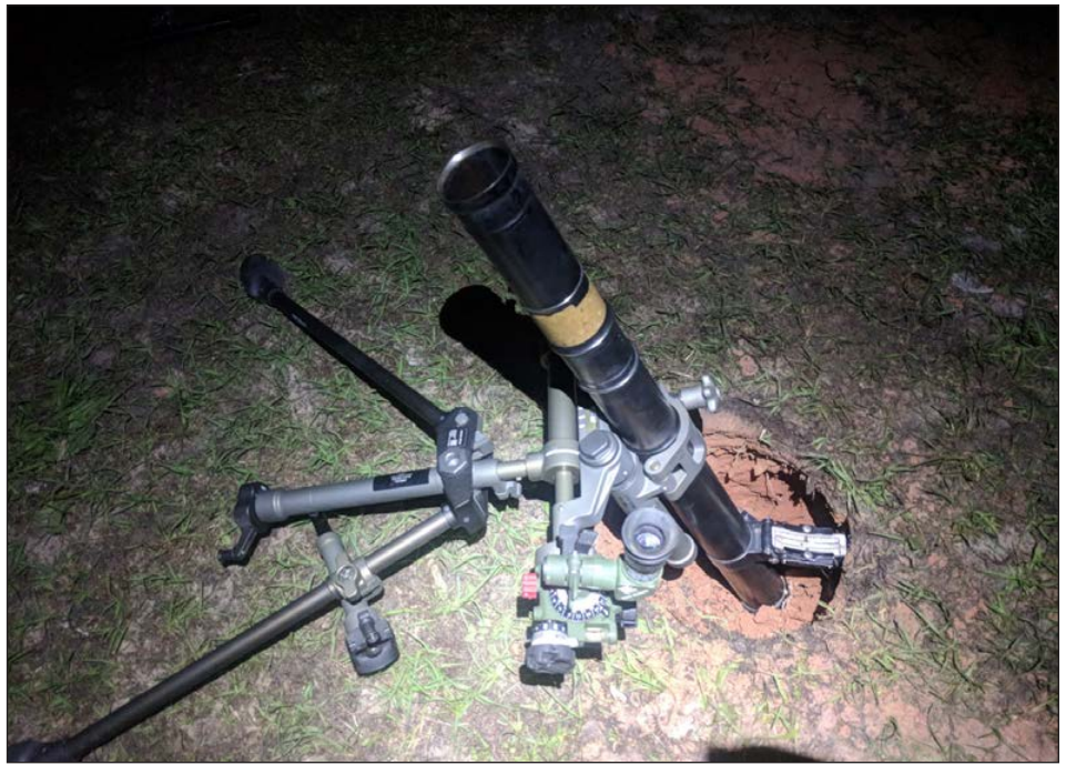
A 60mm mortar base plate digs into the ground due to poor soil conditions.
