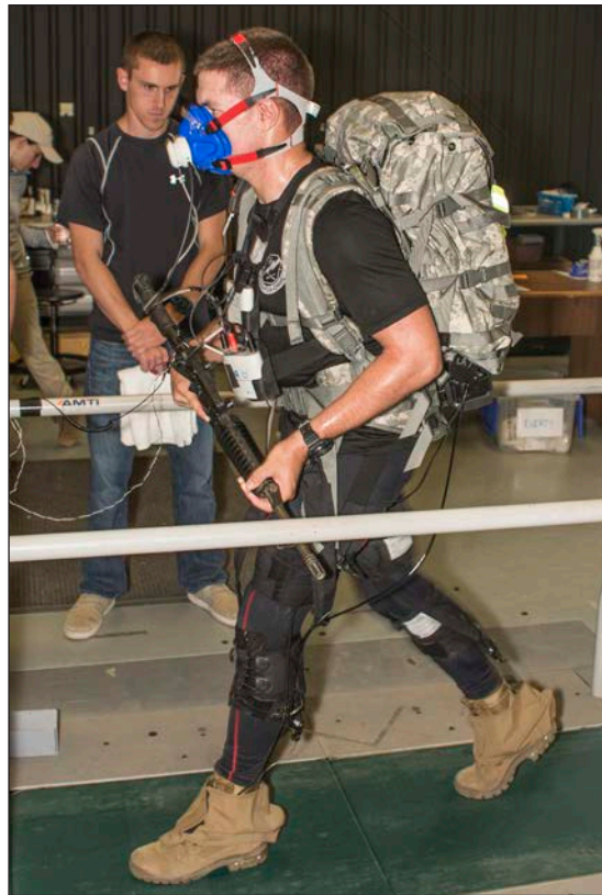
A Soldier wears an exosuit while on a treadmill at a U.S. Army Research Laboratory facility at Aberdeen Proving Ground, MD, on 15 June 2017. The suit is part of the Army's Warrior Web Program. (Photo by David McNally)
