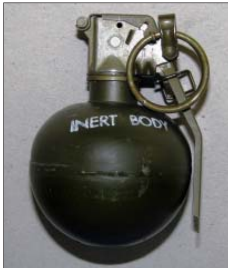
The Confidence Clip, which fits between the grenade fuze and body, securely fastens the pull ring in place to prevent accidental removal or rattling.
