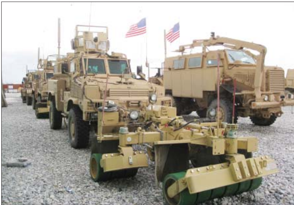
The improved SPARK includes an additional third roller bank and is currently compatible with nearly all military wheeled and tactical vehicles, including all MRAP variations and HMWVs.
