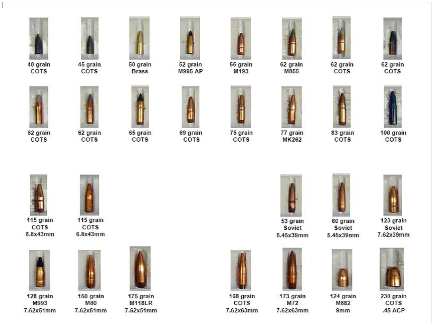
Figure 1 — Original study ammunition configurations (Source: ARDEC)
