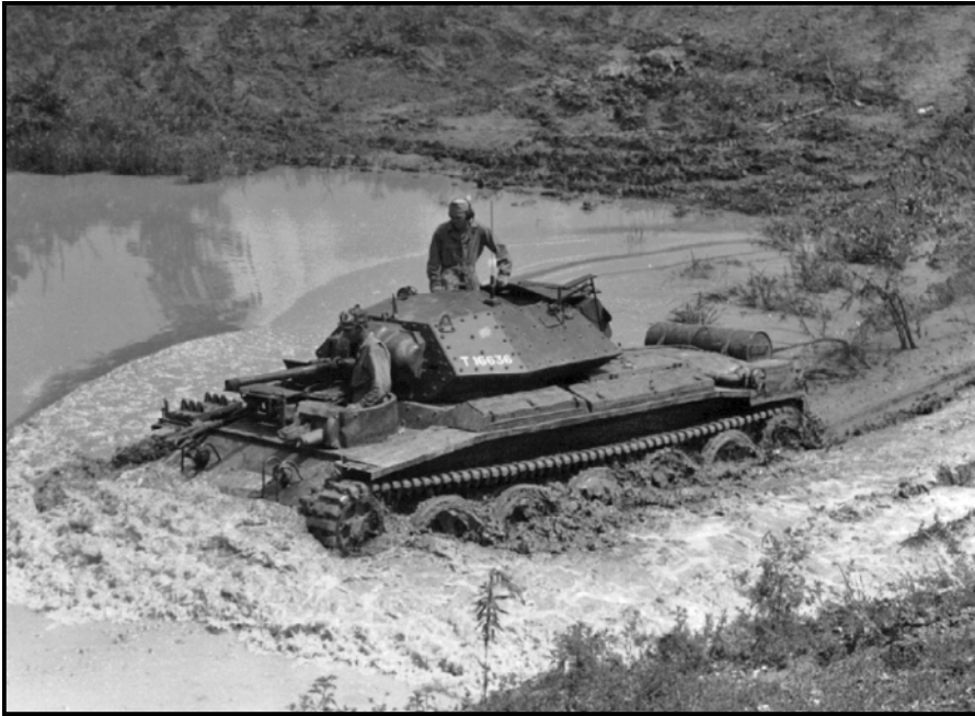
Post-WWI British neglect of tank development handicapped their armored force well into WWII. This Crusader, shown being tested at Fort Knox in 1942, weighed just 18 tons, mounted an ineffective 37mm cannon, and still employed riveted armor, which had been discredited because, when hit, the rivets flew around inside the fighting compartment.
