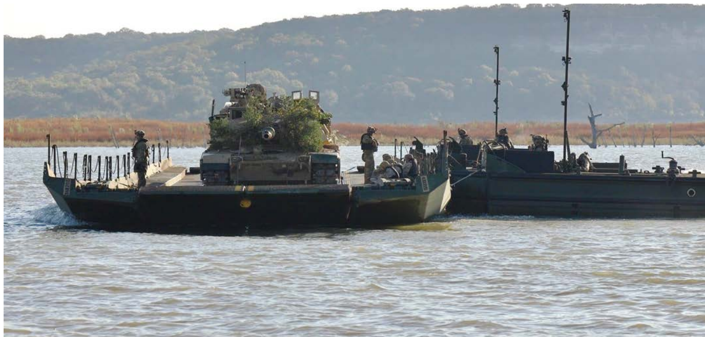
Figure 1. 1/1CD rafting their Armored Cavalry Troop during Remagen Ready 24-01 – An M1 Abrams tank rides on a 43 rd Multi-Role Bridge Company (MRBC) raft under the direction of 2-8 Cavalry and the 20 th Engineer Battalion. Rafting operations took place after 2-5 Cavalry had seized far-side objectives via air and boat assaults. (U.S. Army photo by MAJ Garrison Spencer, U.S. Army Corps of Engineers (USACE) Public Affairs Officer)
