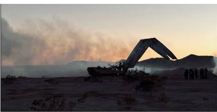
Figure 3. Army engineers deploy a JAB. (U.S. Army photo by CPT Galen King)
