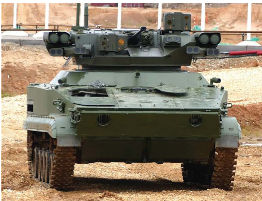
Figure 1. A Russian UGV based on the BMD armored chassis. Russia’s armed forces will likely integrate UGVs with motor rifle battalions because of the Ministry of Defense’s “Weapons Robotizing 2015” program.
