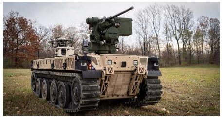
Figure 1. The RCV-Light can be equipped with a tethered unmanned aerial system, a small drone that can be deployed to conduct aerial reconnaissance while the vehicle is at a safe distance. Other equipment to be tested on the RCV-Light experimental prototype includes the M153 Common Remotely Operated Weapons Station II (CROWS II), the .50 caliber M2 machinegun and the 40mm MK19 Mod 3 automatic grenade launcher. (Photo by Bruce Huffman, Michigan National Guard)
