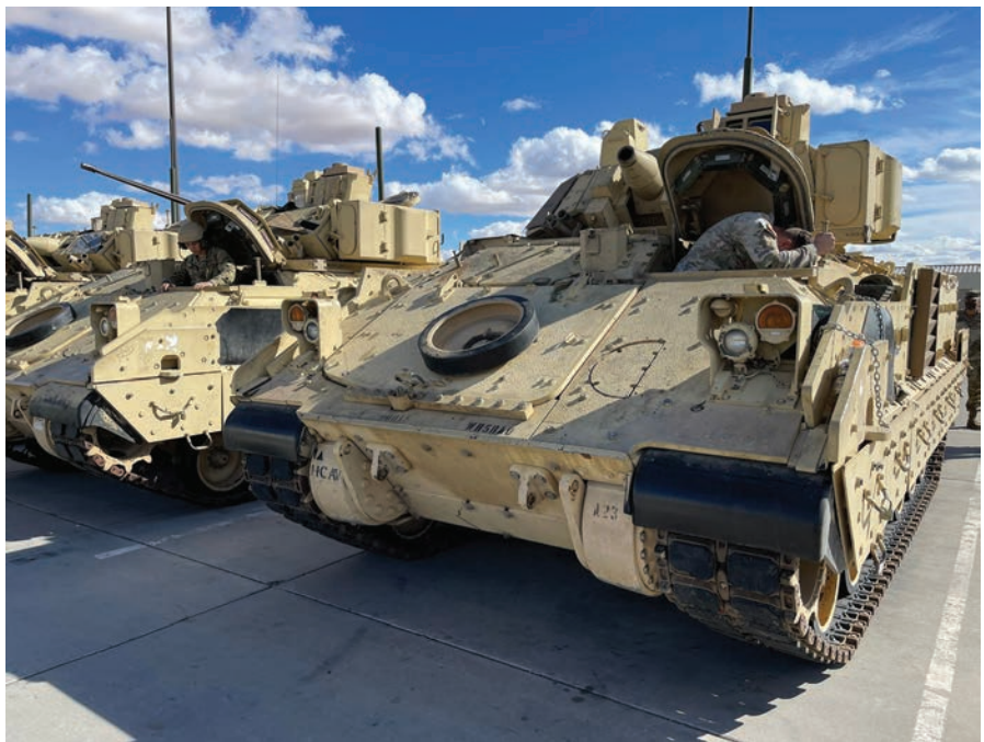
Figure 1. Troopers from 1 st Squadron, 1 st Cavalry Regiment, conduct PMCS on their M2A3 Bradleys at Fort Bliss, TX. (Photo by MAJ Steve Modugno, 2 nd Brigade Combat Team, 1 st Armored Division, Public Affairs)
