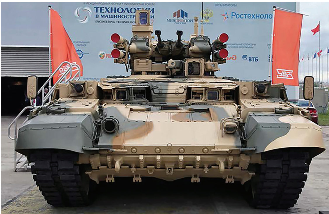
Figure 5. The first model of BMPT-72. Note the unarmored ATGM tubes, hull-mounted grenade launchers above the tracks and Active Protection System tubes barely visible at the base of the turret. (Photo copyright Vitaly Kuzmin. Licensed under a Creative Commons Attribution-NonCommercial-NoDerivatives 4.0 International License.)
