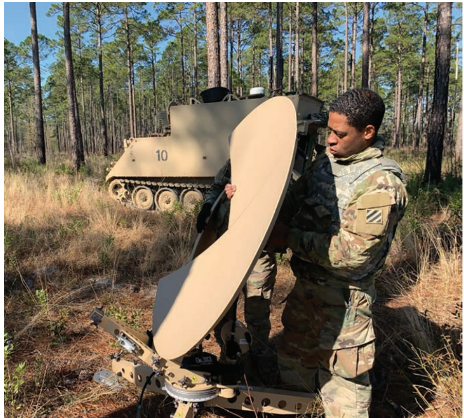
Figure 2. Soldiers assigned to the Can-Do Battalion, 3 rd Battalion, 15 th Infantry Regiment, 2 nd ABCT, 3 rd Infantry Division, set up a satellite terminal to test and assess one of the three commercial OTM network equipment sets during the U.S. Army's three-week armored-formation OTM network pilot at Fort Stewart, GA, Feb. 2, 2022. (U.S. Army photo by CPT Detrick Moore)
