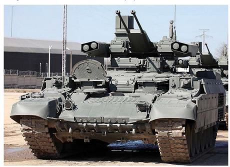
Figure 1. The Russian army's BMPT-72. The turret has been modified from earlier models, with armor surrounding the ATGM tubes and some other changes, but the hull retains the grenade launchers. (Photo copyright Vitaly Kuzmin. Licensed under a Creative Commons Attribution-NonCommercial- International License NoDerivatives 4.0.)
