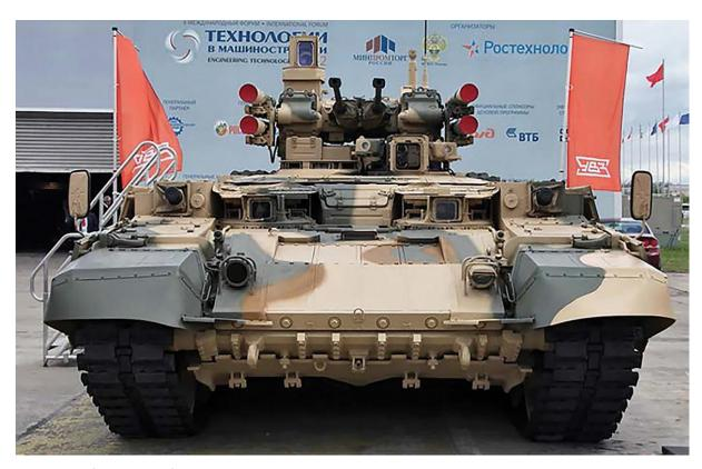
Figure 5. The first model of BMPT-72. Note the unarmored ATGM tubes, hull-mounted grenade launchers above the tracks and Active Protection System tubes barely visible at the base of the turret. (Photo copyright Vitaly Kuzmin. Licensed under a Creative Commons Attribution-NonCommercial-NoDerivatives 4.0 International License.)
