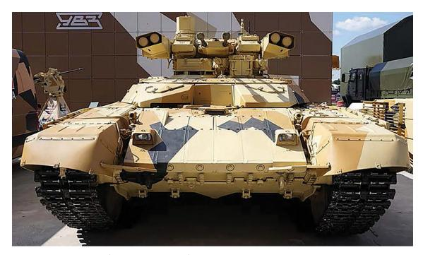
Figure 7. The latest model of BMPT-72 destined for the export market. Note the redesigned turret and lack of forward-facing grenade launchers. (Photo copyright Vitaly Kuzmin. Licensed under a Creative Commons Attribution-NonCommercial-NoDerivatives 4.0 International License.)
