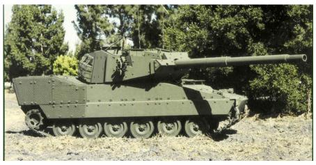
Figure 2. M8 Armored Gun System (AGS) Level 2 armor, circa 1994. (U.S. Army photo)
