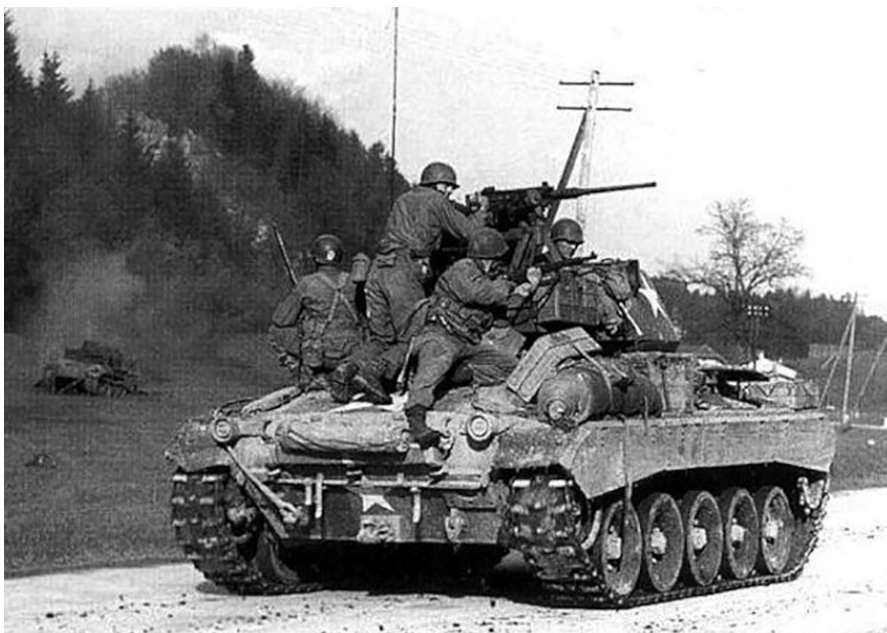
Figure 1. An M24 Chaffee light tank belonging to 106 th Cavalry Group moves on the outskirts of Salzburg, Austria, in May 1945. The M24 was a Johnny-come-lately to the war effort, but armored-division crews reported liking the Chaffee's improved off-road performance and reliability. However, they were most appreciative of the 75mm main gun, which was a vast improvement over the M5A1 Stuart tank's 37mm gun. In spite of the gun's upgrade, cavalry was still unable to perform its historic and traditional mission in Europe and the following conflict, Korea.
