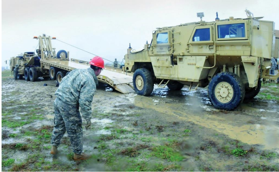
Figure 4. SGT Jeffrey Palmer, an instructor, keeps a careful watch as students in the MCRS module of the H8 Recovery Specialist Course pull a disabled mine-resistant ambush-protected vehicle onto the MCRS' tilt-deck recovery trailer during training at Downer Range, Fort Lee, VA. The H8 course is a three-week additional-skill identifier course at Fort Lee. (U.S. Army photo)
