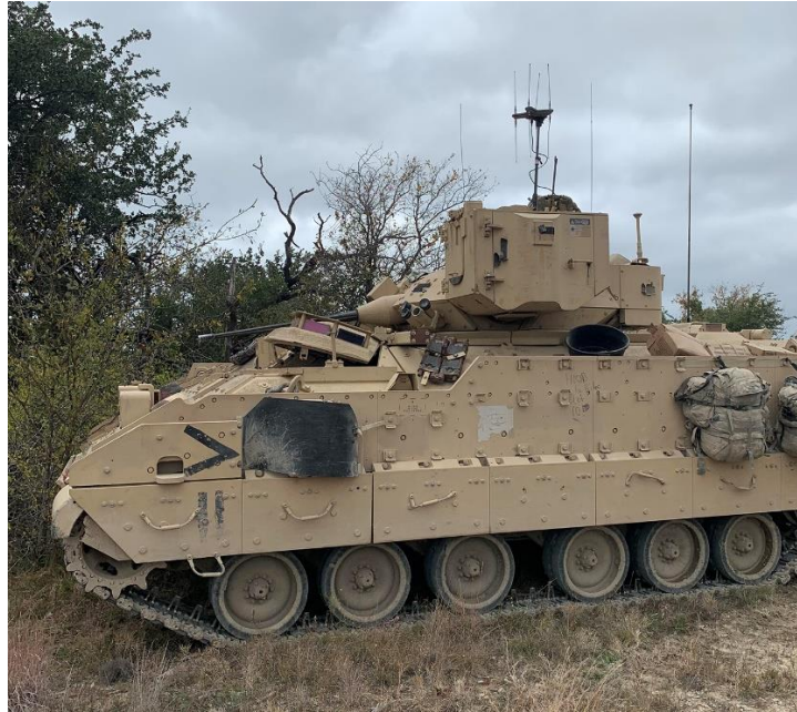
Figure 6. VROD mounted on the Wild Bill BFIST in a collection site.
