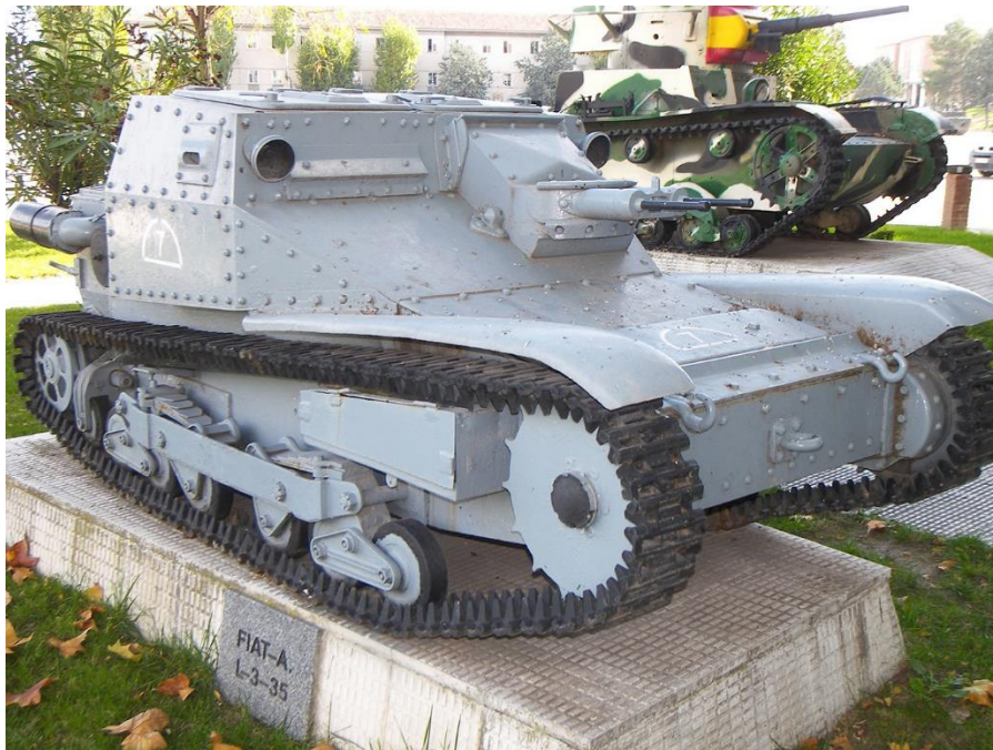
Figure 2. This is the Italian light tank Fiat L-3 CV 35 made by Fiat-Ansaldo. A total of 155 tanks were provided by Fascist Italy to Nationalist Spain. The first L-3 tanks arrived in Spain in late August 1936, the first modern tanks entering service in the Spanish Civil War. Outgunned – they were armed with only two fixed machineguns – they were not a match to Soviet tanks. They did not even have a turret; to aim the machineguns, the whole tank had to move. Some 60 Italian tanks survived the war and even continued in active service until the early 1950s in Spanish cavalry units. (Author's collection)
