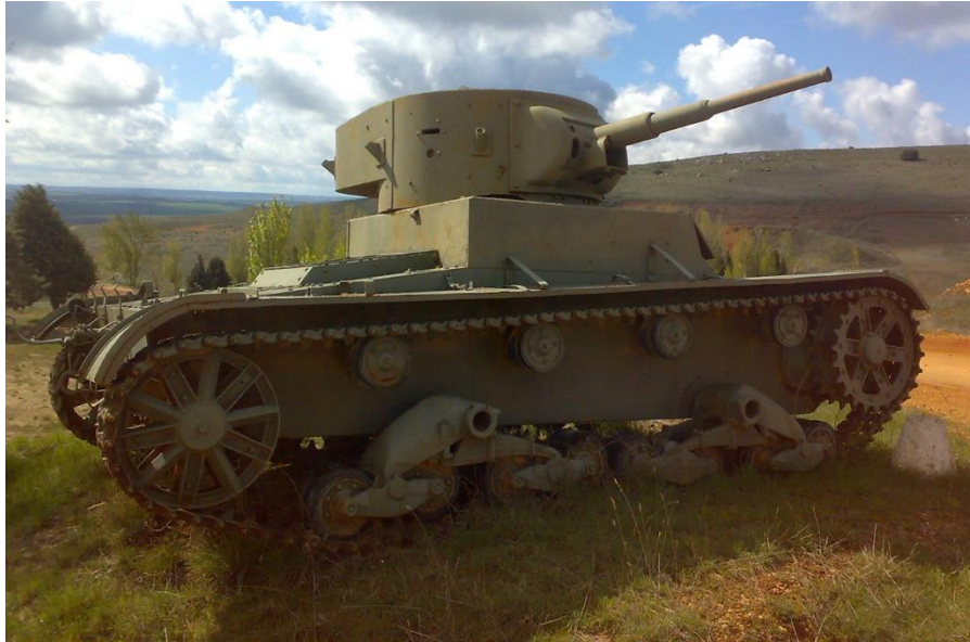
Figure 4. This is a T-26B Soviet light tank furnished by the Soviet Union. Those tanks started to arrive into Republican Spain in October 1936 and were real tanks with a main gun and machineguns. They were heavier than the ones provided by Germany and Italy to Nationalist Spain and better protected. The Soviet Union provided 286 T-26B tanks to the Spanish Popular Army, and more than 130 ended up in the service of the Nationalist Army by the end of the war. They remained in active service until the early 1950s. This picture was taken near a memorial for the civil war on what was once the battlefield of the Ebro, which took place in 1938.
