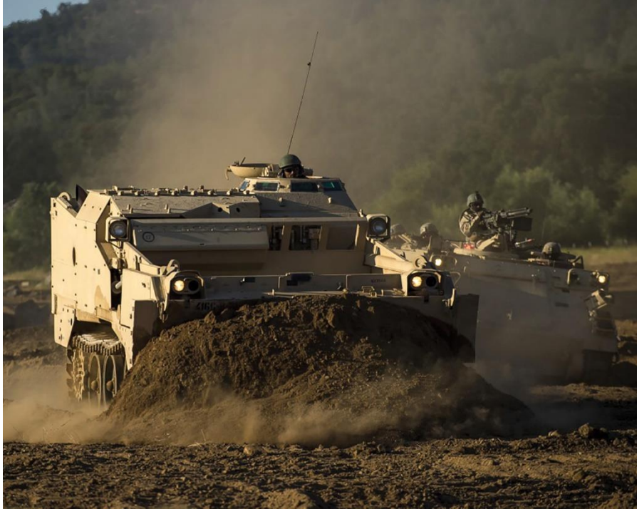
Figure 3. U.S. Army Reserve combat-engineer Soldiers use an M-9 Armored Combat Earthmover to clear dirt for a combined-arms breach during a CSTX at Fort Hunter Liggett, CA, July 22, 2018. (U.S. Army Reserve photo by MSG Michel Sauret)
