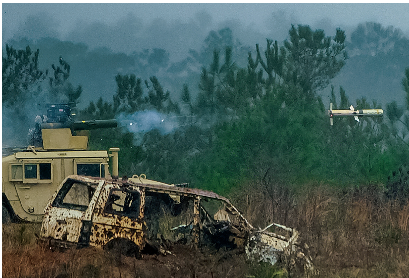
Figure 1. Soldiers of the 316 th Cavalry Brigade's Heavy Weapons Leaders Course fire for qualification on the vehicle-mounted tube-launched, optically tracked, wire-guided anti-tank missile system at Cactus Range, Fort Benning, GA. (Photo by Patrick A. Albright, Maneuver Center of Excellence Public Affairs photographer)
