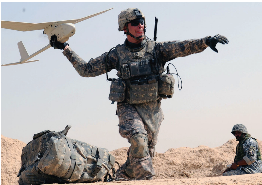
Figure 1. An RQ-11B Raven, an SUAS employed by 2/2 Cav, is launched by a Soldier in Iraq. (U.S. Army photo)
