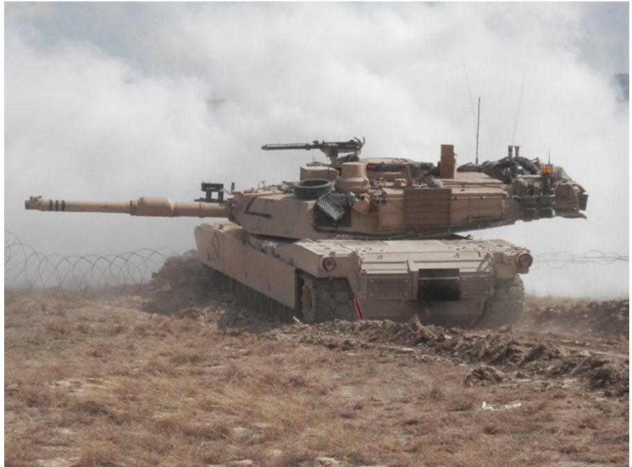
Figure 5. A plow tank from Dragoon Company conducts a breach during a platoon STX. Note the loaded vehicle smoke grenades. (Photo by COL Esli Pitts)
