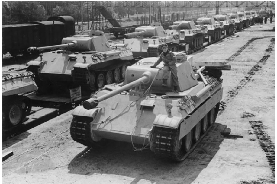
Figure 4. A Panther moves toward its assigned railcar. The Panther's lack of range severely limited its operational mobility, and it often had to rely on railcars if moving farther than 100 kilometers.
