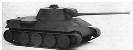
Figure 2. A wooden model of Daimler-Benz's recommended version for the Mark V Panther. The prototype was named VK3002 and had some clear similarities to the Soviet T-34 tank.
