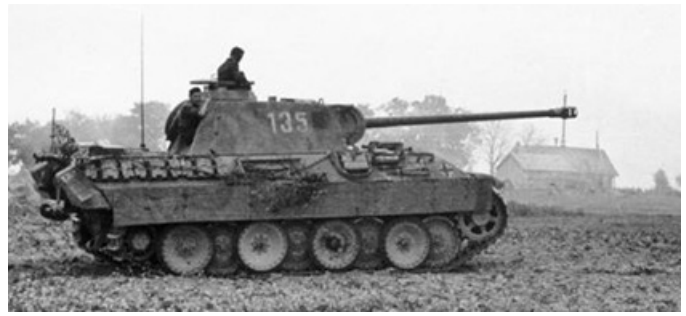
Figure 3. Panther with full Schürzen spaced armor attached, intended to supplement the side armor above the large wheels.
