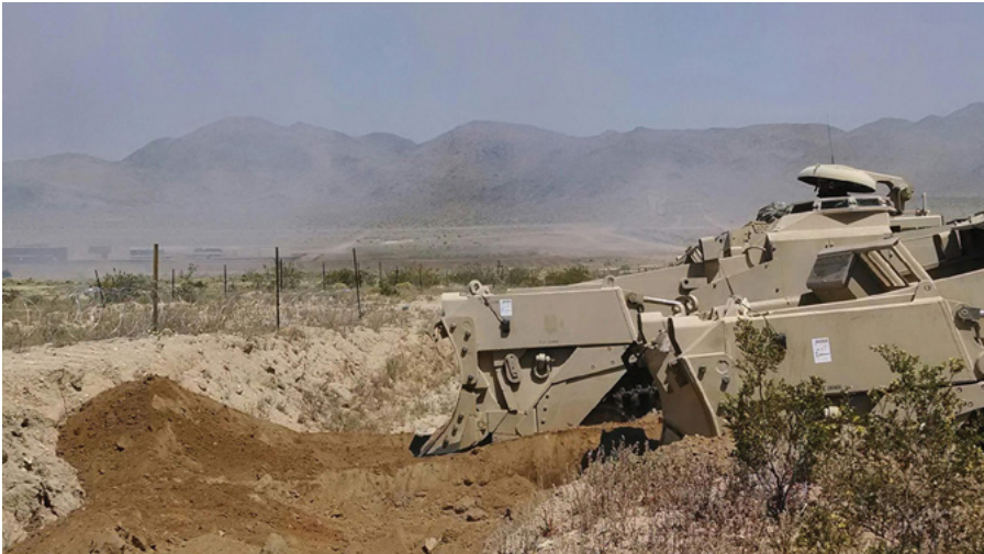
Figure 3. An Armored Combat Earthmover fills a ditch. Engineering assets like this one are of high value to enemy forces. (Photo by CPT John Barrington)
