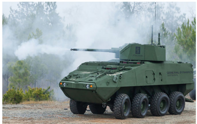
Figure 3. A prototype Stryker vehicle with 30mm-gun turret. (Photo courtesy of General Dynamics)
