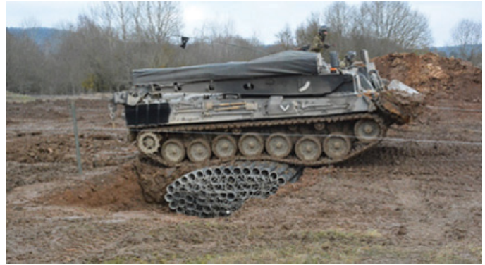
Figure 2. A Leopard engineer tank crosses the gap after engineers emplace the fascine.
