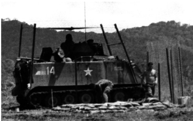
Figure 3. An M113 behind chain-link fencing intended to prematurely detonate incoming RPG rounds.
