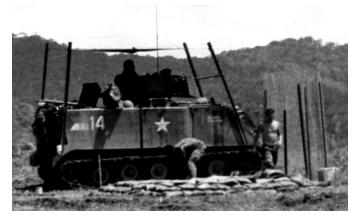
Figure 3. An M113 behind chain-link fencing intended to prematurely detonate incoming RPG rounds.
