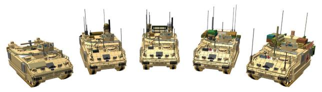
Figure 9. Artist depiction of the AMPV variants. From left to right, they are the mortar carrier, general-purpose, mission command, medical evacuation and medical treatment vehicles.
