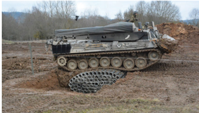
Figure 2. A Leopard engineer tank crosses the gap after engineers emplace the fascine.
