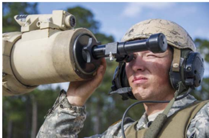
Figure 2. SPC Cody Winder, an M1A2 System-Enhancement Program Abrams loader for 2 nd ABCT, 3 rd Infantry Division, conducts bore-sighting procedures during live-fire accuracy screening. (Photo by SGT Richard Wrigley)
