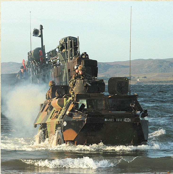
Figure 3. An AMX10 RC used by the French 1st Régiment de Spahis in January 2006. The vehicle's missions are armored reconnaissance, armored support and flanking security.
