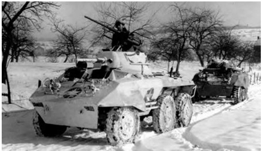
Figure 1. During the winter of 1944-1945 in the ETO, vehicles were camouflaged with white paint for use in snow conditions. Here the lead M8 Greyhound armored car has been painted, while the following M8 has not.
