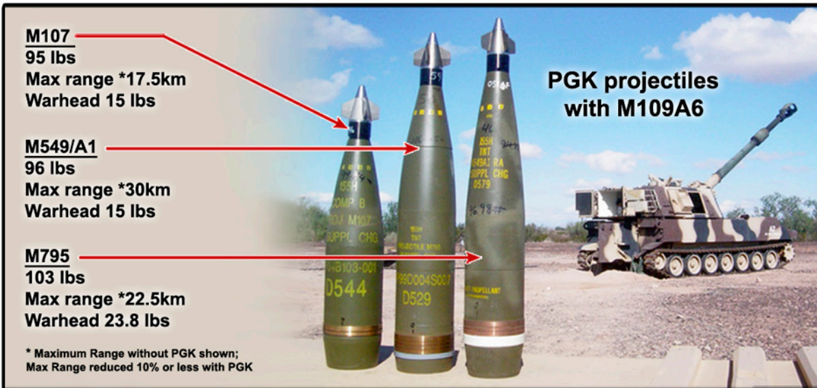
Figure 2. Options of artillery ammunition to precisely combat the target.
