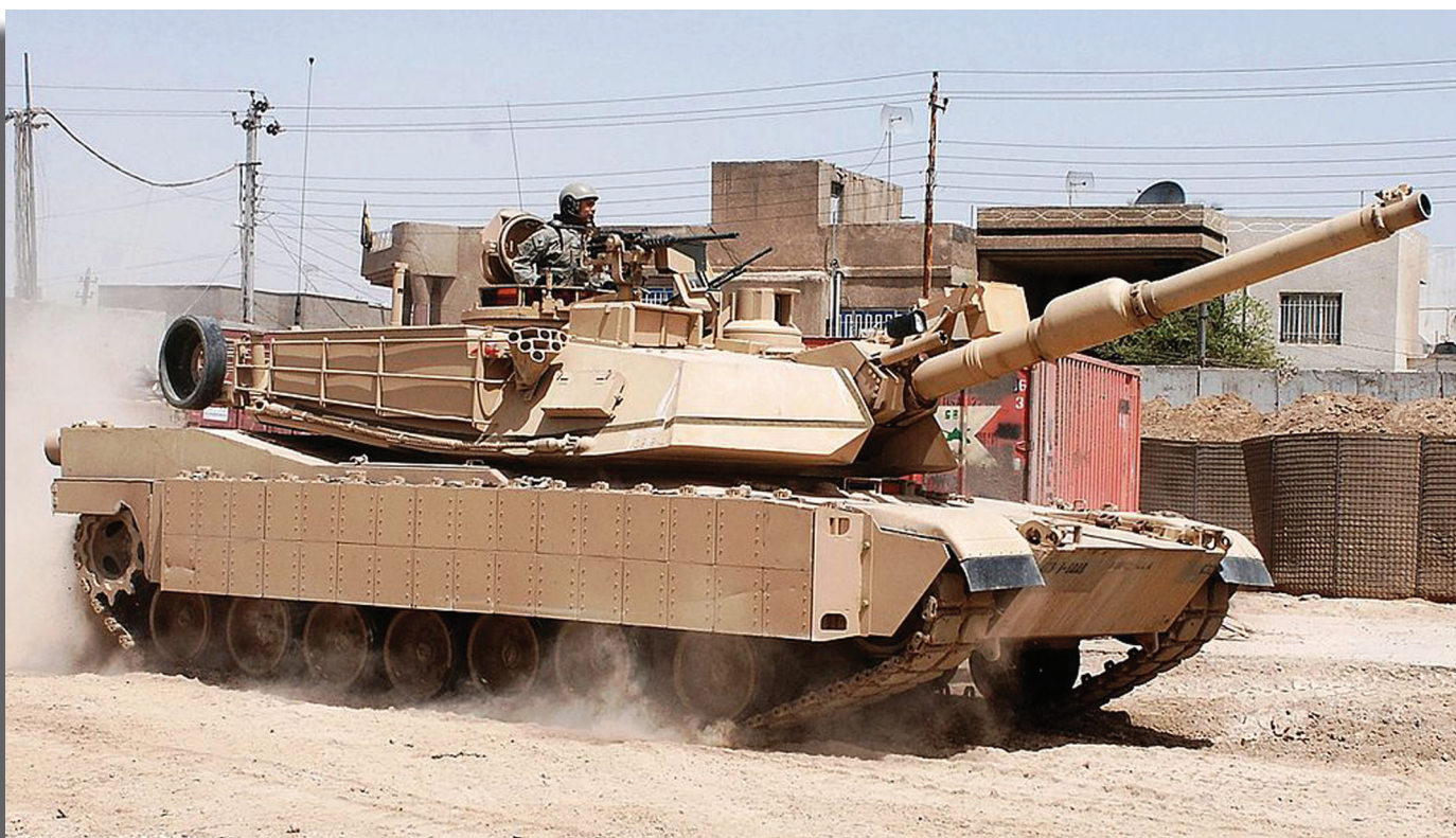
An M1A2 System Enhancement Package (SEP) Abrams with Tank Urban Survival Kit (TUSK) and Mounted Soldier System (MSS) in Iraq.
